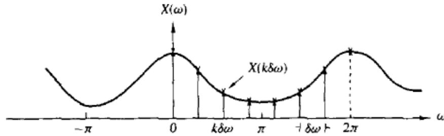
Figure 5.1 Frequency-domain sampling of the Fourier transform.
