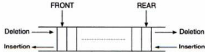
Figure 5.9 A deque structure.
