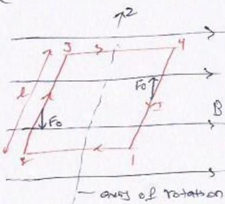
The  $d\vec{I}$  is parallel to  $\vec{B}$  along sides 12 and 34 of the loop and no force is exerted on those sides. (9)
