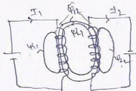
The flux  $\Phi_{12}$  is the flux passing through circuit 1, due to current  $I_2$  in circuit 2. If  $B_2$  is the field due to  $I_2$  and  $S_1$  is the area of circuit 1, then
