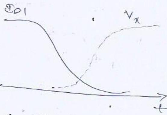
fig: Condition to ensure minimal overlap in drain current and voltage.
