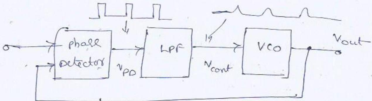
fig(2) Addition of low pass filter to remove high frequency components generated by Phase detector.
