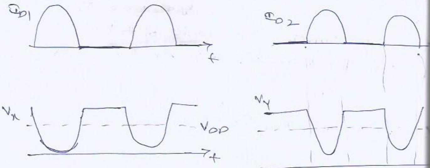
Fig 2: Current and Voltage waveforms in a class B stage.
