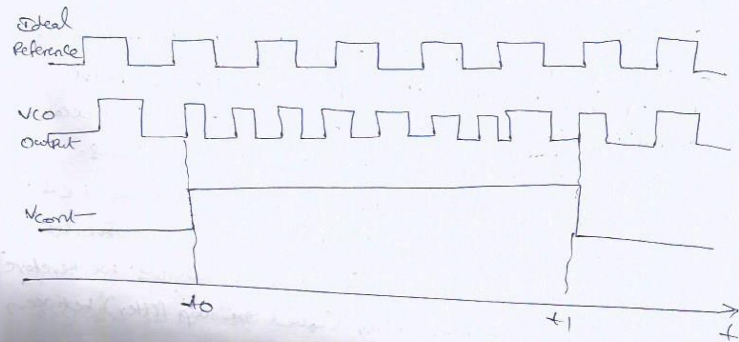
fig. Alignment of vco output phase by changing its frequency.
