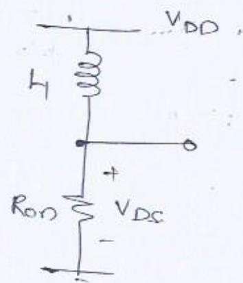
fig: o/p stage with switching transistor.
