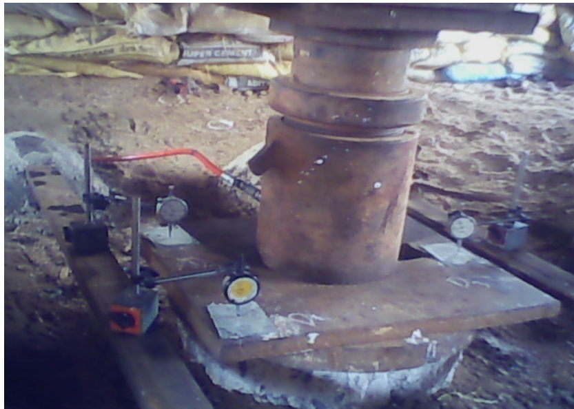
Fig. 7.4(b): Pile load Test Setup
