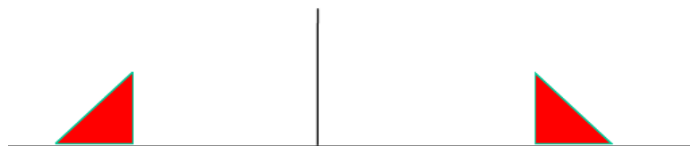
Figure .2 : Spectrum of the SSBSC wave
