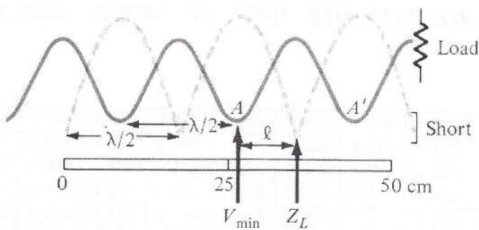
(b) Determining the location of the load  $Z_L$  on a slotted line
