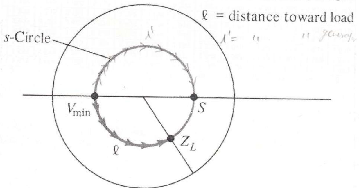
And also locate the load by using  $l'$ , which is the distance of  $V_{min}$  toward the generator. Either  $l$  or  $l'$  may be used to locate  $Z_L$ .
