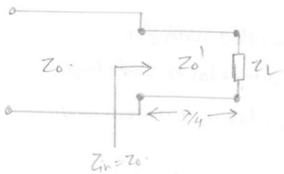
Load matching using a  $\frac{1}{4}$  transformer.
