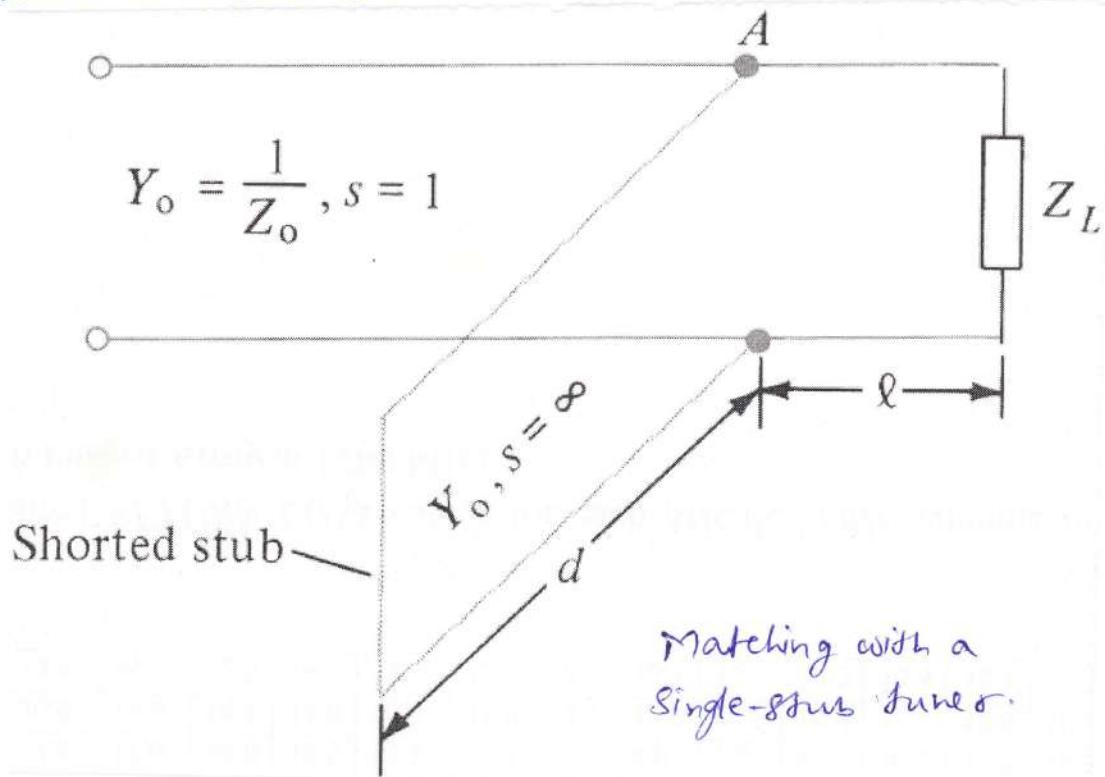
The stub has the same characteristic impedance as the main line. It is more difficult to use a series stub although it is theoretically feasible. An open circuited stub radiates some energy at high frequencies. Consequently, short-circuited parallel stubs are preferred.
