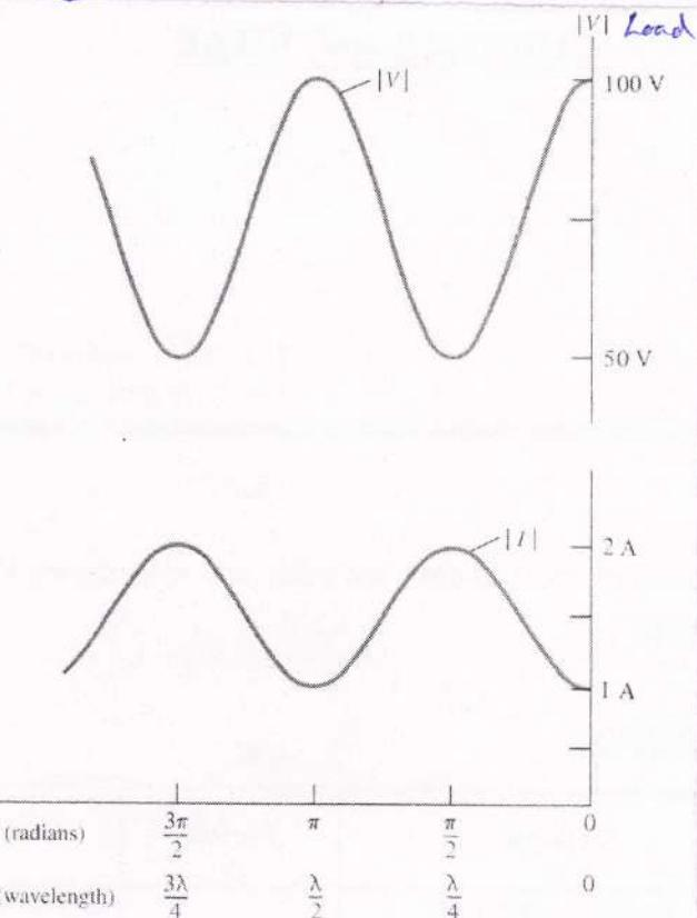
Fig: Voltage & Current wave patterns on a lossless line terminated by a resistive load.
