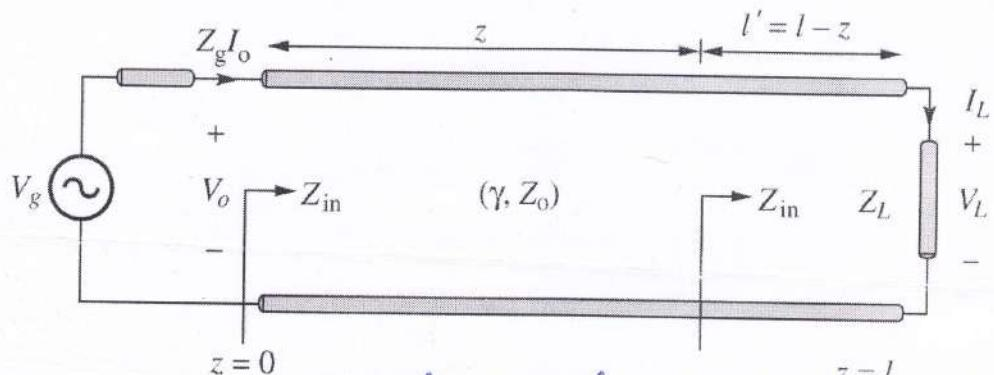
(a) Input impedance due to a line terminated by a load.
