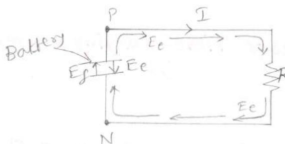
A Circuit Showing Emf-Producing field  $E_f$  & electrostatic field  $E_e$
