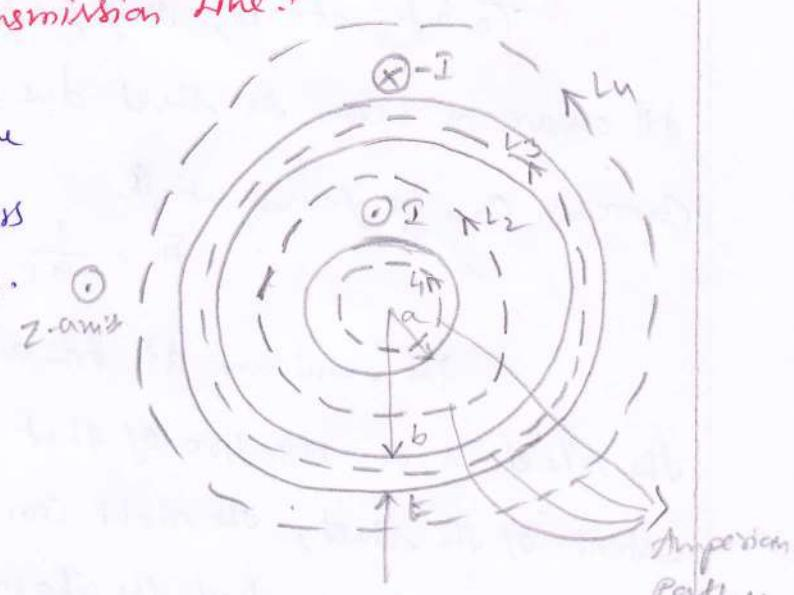
Cross section of the transmission line, the positive  $\hat{z}$ -direction is out of page.
