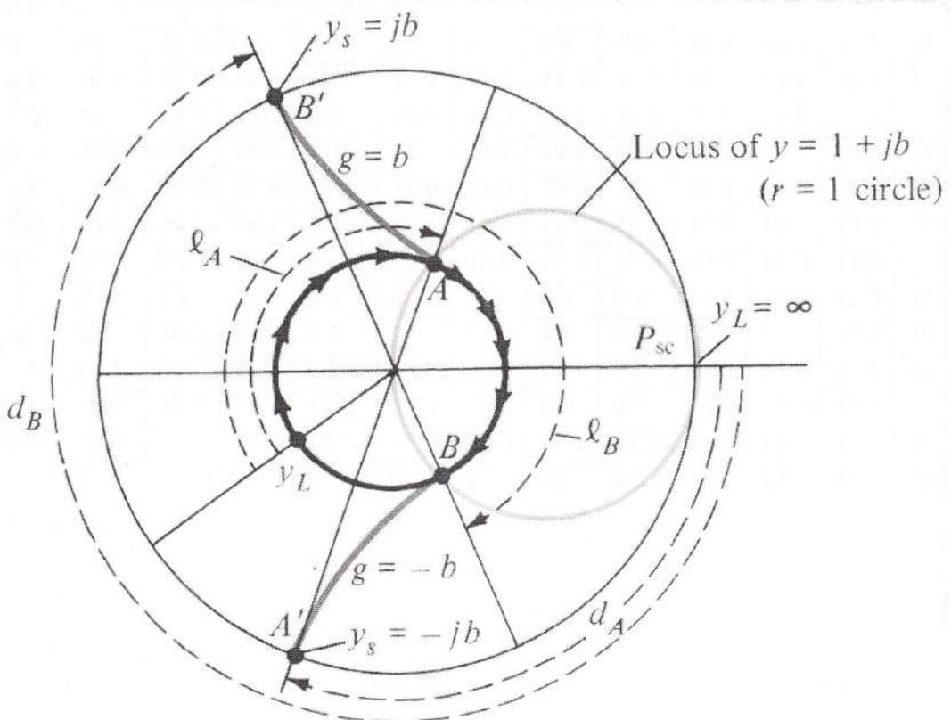
Using the smith chart to determine  $l$  &  $d$  of a shunt loaded single-stub tuner.
