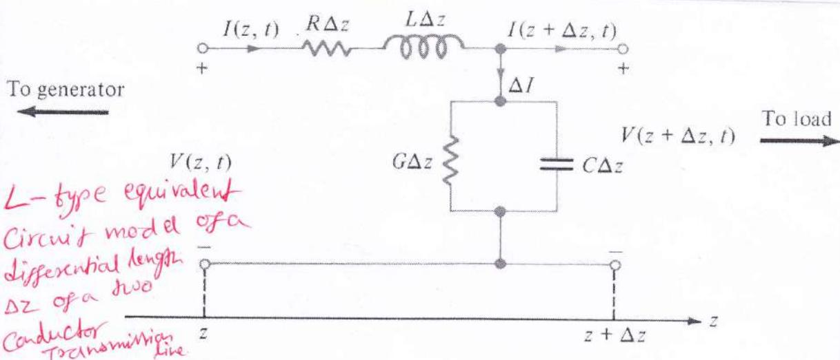
Let us consider an incremental portion of length  $\Delta z$  of a two-conductor transmission line. The model of the equivalent circuit shown in figure, the line parameters are  $R, L, G, C$ .
