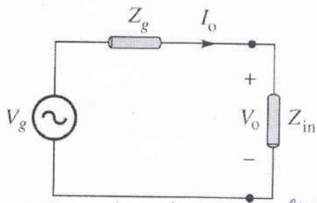
(b) Equivalent circuit for finding  $V_o$  &  $I_o$  in terms of  $Z_{in}$  at the input.
