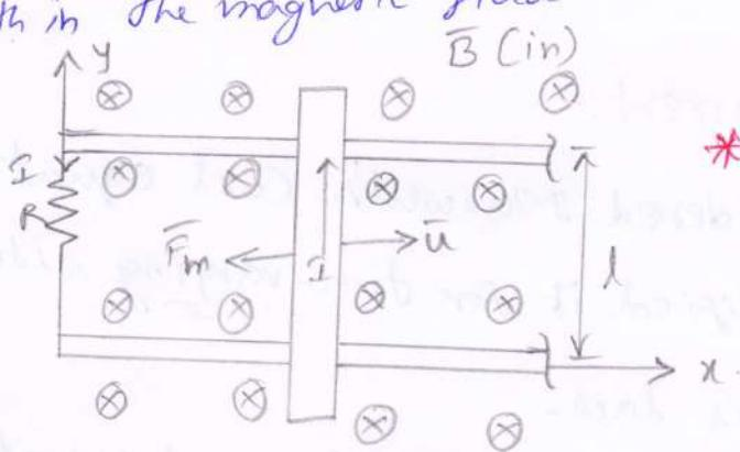
Consider the voltage is generated as the coil rotates within the magnetic field. Consider a rod is moving between a pair of rails. In this  $\bar{B}$  &  $\bar{u}$  are perpendicular, then the force is,
