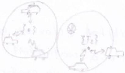
The user who starts a call in one zone has to reinitiate the call when moving into a new zone because the call will be dropped. This is an undesirable radio telephone system since there is no guarantee that a call can be completed without a handoff capability.
