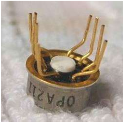
The metal can (TO) Package
