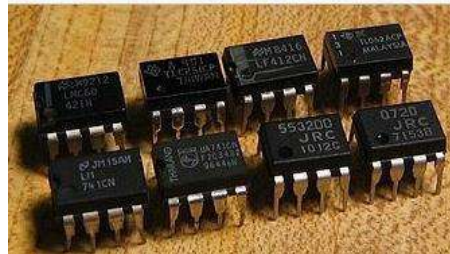
The Dual-in-Line (DIP) Package
