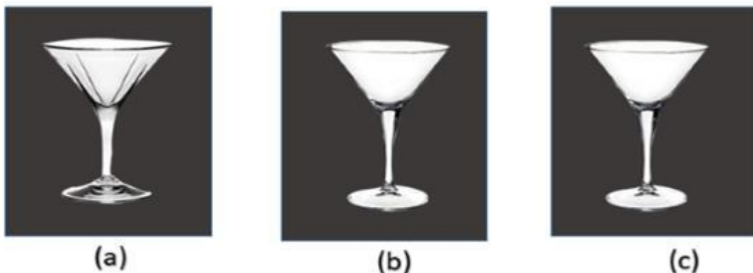
Fig: A Polygon mesh approximation of an object (a) is rendered with flat shading (b) and With Gouraud shading (c)
