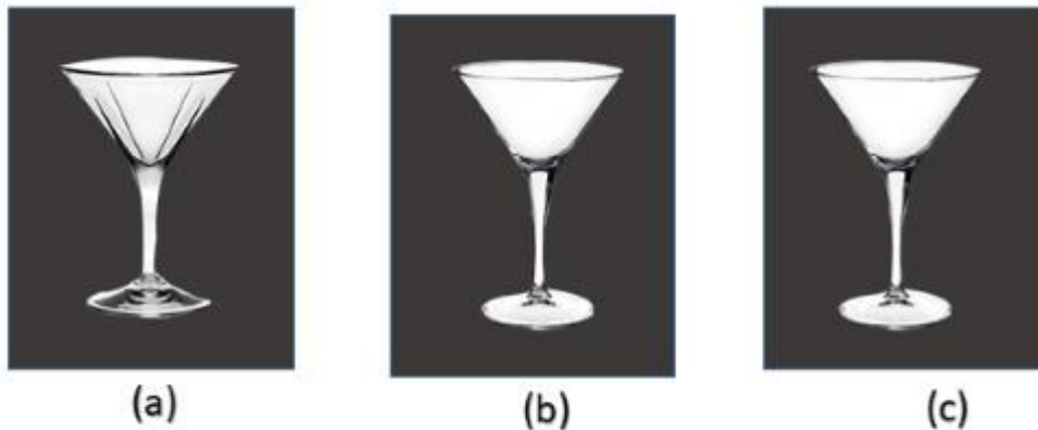
Fig: A Polygon mesh approximation of an object (a) is rendered with flat shading (b) and With Gouraud shading (c)
