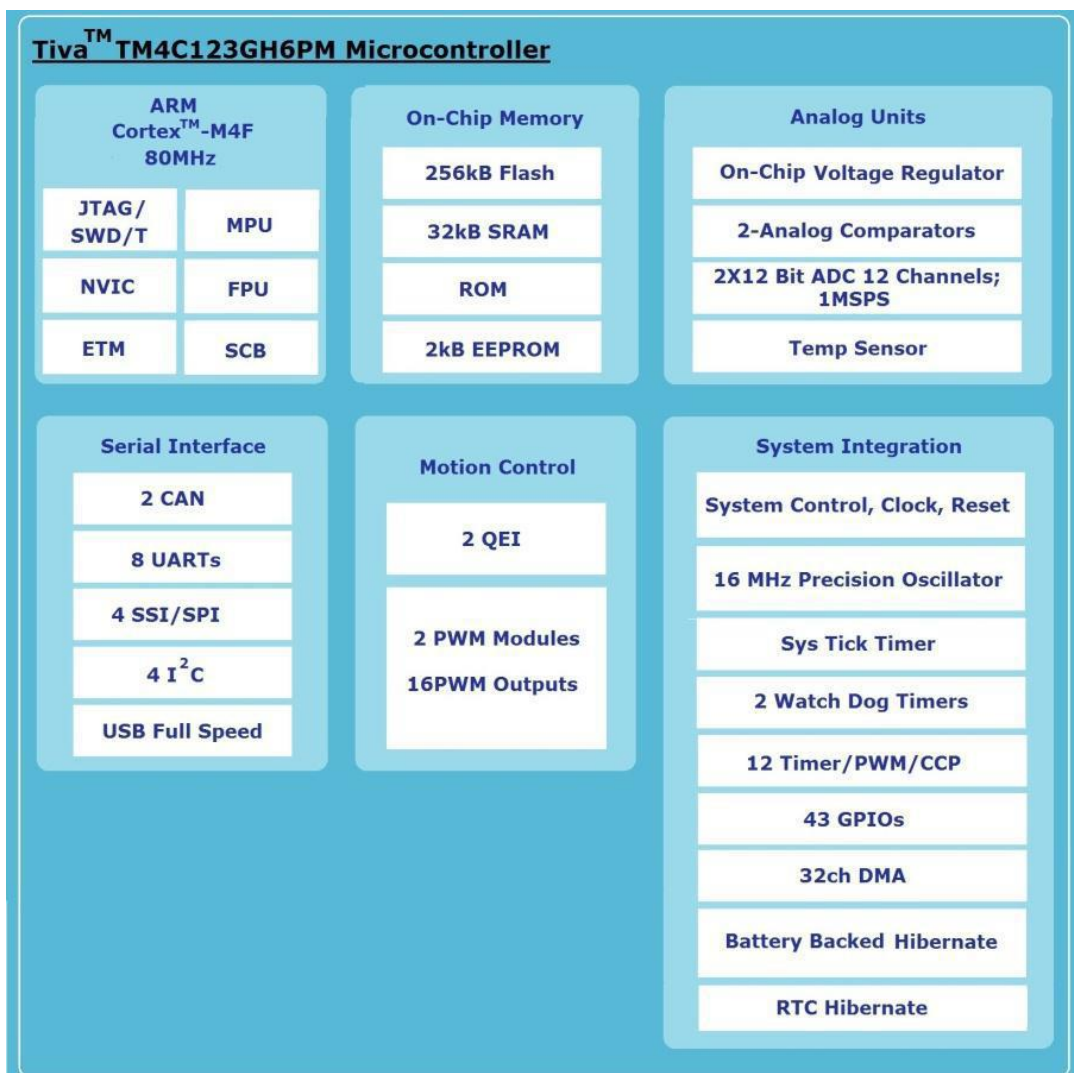
Fig 5: TM4C123GH6PM Microcontroller Block Diagram
