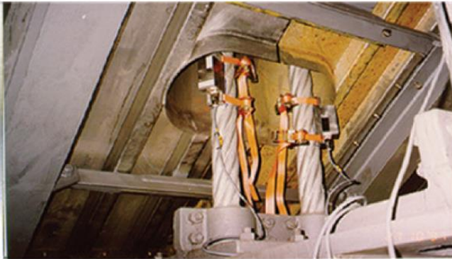
Figure Accelerometers used in vibration monitoring of civil engineering structures.
