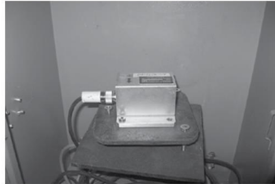
Figure Accelerometers used in vibration monitoring of civil engineering structures.
