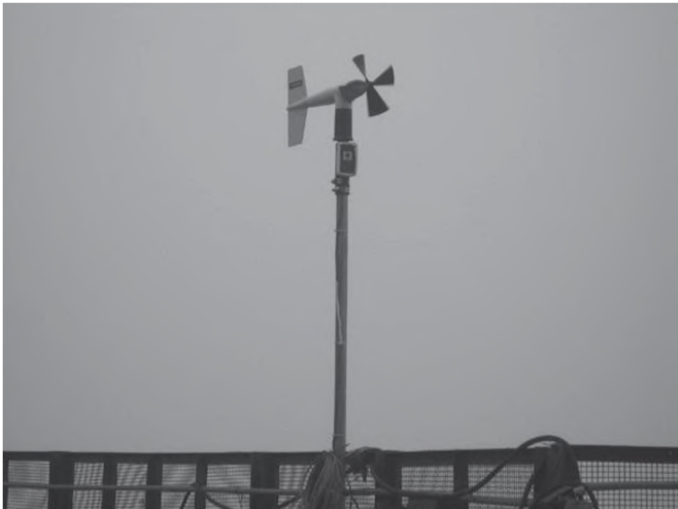
Figure 5 Anemometer (R.M. Young Model 05103L) installed on Canton Tower.
