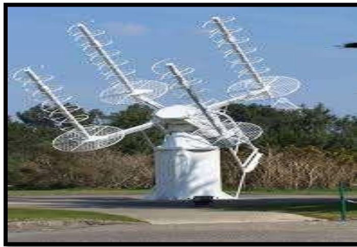
Fig 2.5: Helical antenna system
