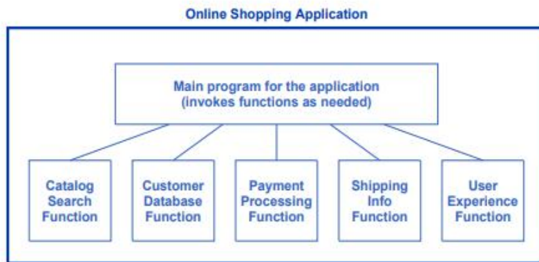
Figure 12.1 Illustration of a monolithic application with all the functions needed to support online shopping built into a single program.
