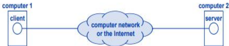
Figure 14.1 An example of traditional client-server communication.
