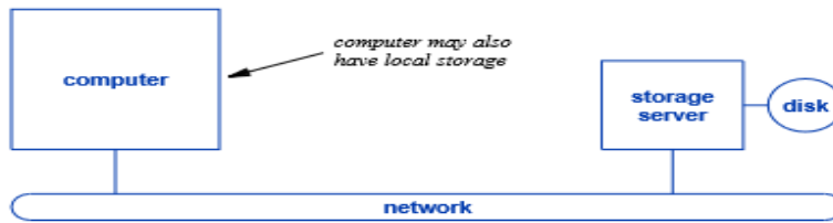
Figure 8.3 Conceptual organization of a remote storage facility with a computer accessing a storage server over a network and disk storage attached to the storage server.
