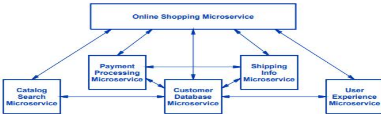
Figure 12.2 Illustration of the shopping application disaggregated into a set of microservices that communicate with one another.
