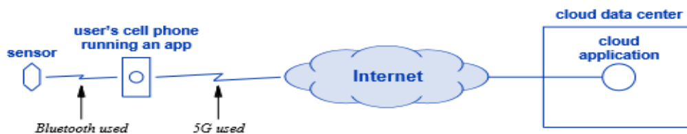
Figure 16.2 An app on a user's cell phone that gathers information from a sensor and sends the information to an application running in a cloud data center for analysis.
